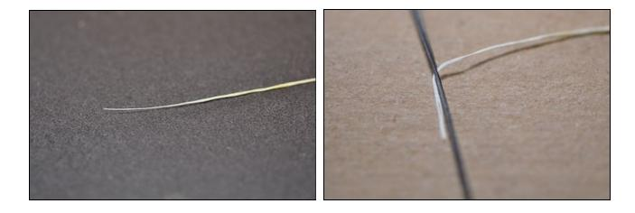
Fig. 3: retwisted plies with coad applied
