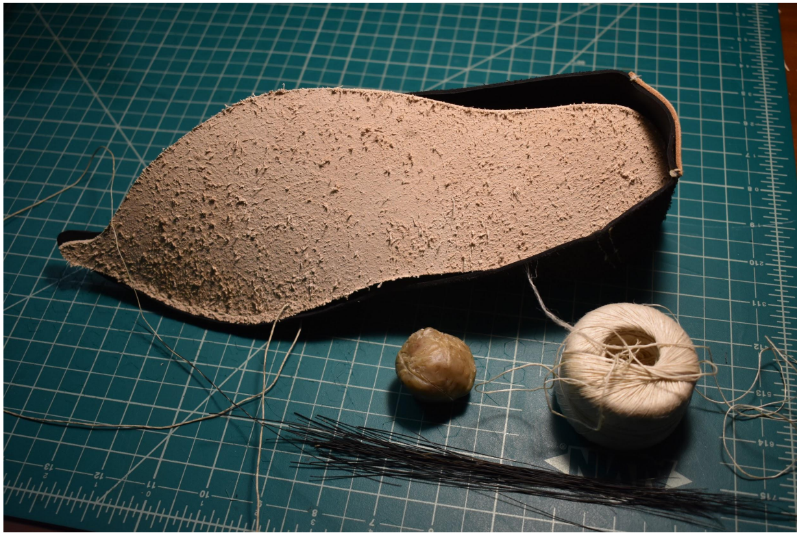
Still life of shoe assembly in progress, boar's bristles, waxed ends, ball of coad, and vintage linen thread.
