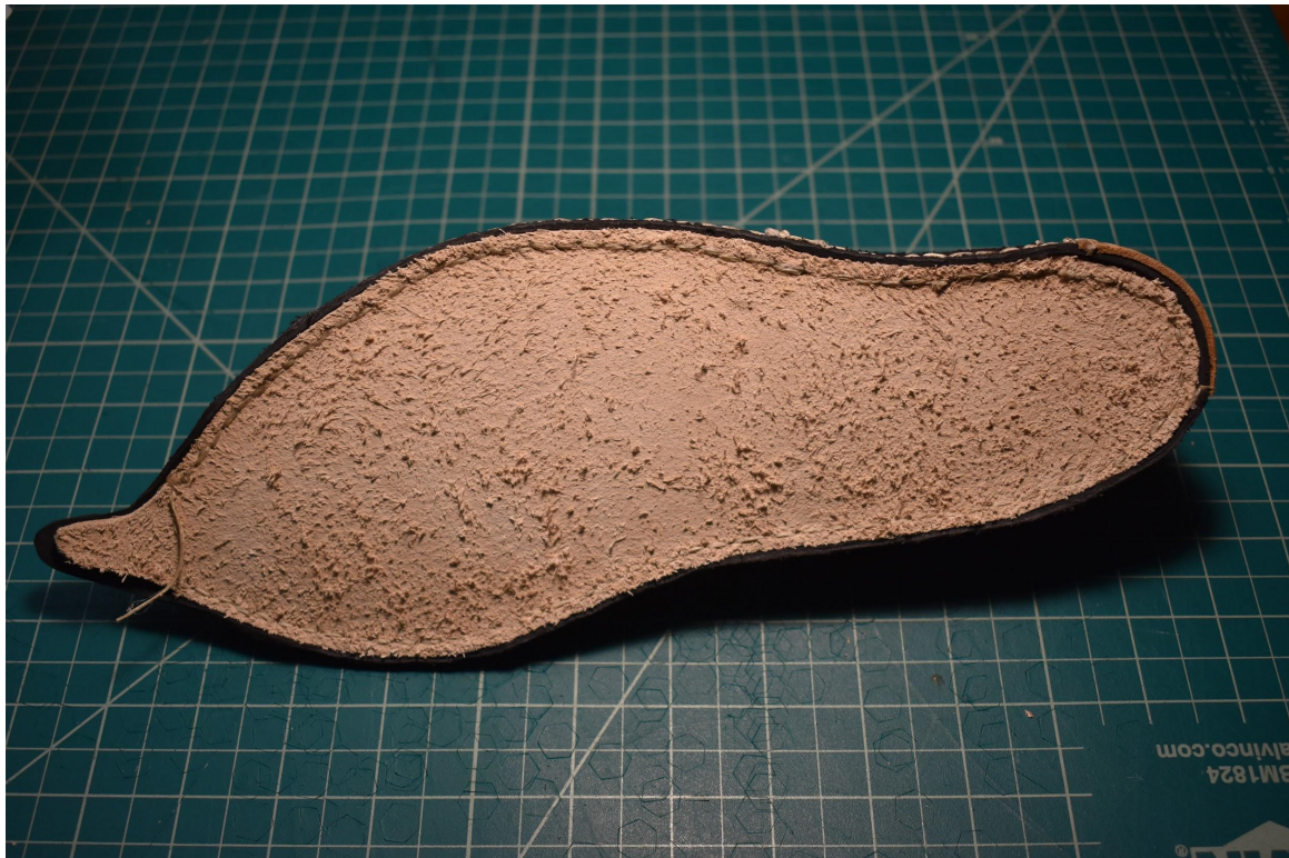
Shoe ready to turn. Note the toe will be left unstitched and closed later because long points such as this one cannot be turned.
