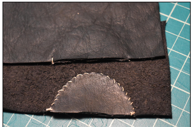
A shoe upper with its side seam stitched closed and the heel stiffener added by whip-stitching the leather through the stiffener but staying within the thickness of the upper’s leather (left). A heel stiffener viewed from the inside and from the outside (right). Not all shoes had heel stiffeners, but this one did so it was added for this project.
