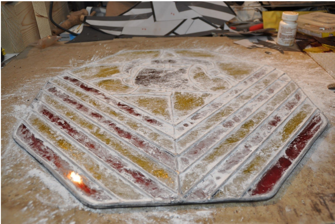
Whiting powder applied as a way to clean the putty by brushing it off.
