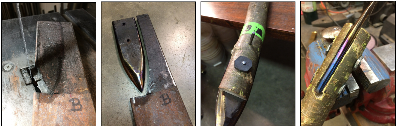
Crafting the custom blade: cutting from found spring steel; cut, ground, polished, and drilled ready to mount; mounting in progress; successfully mounted.
