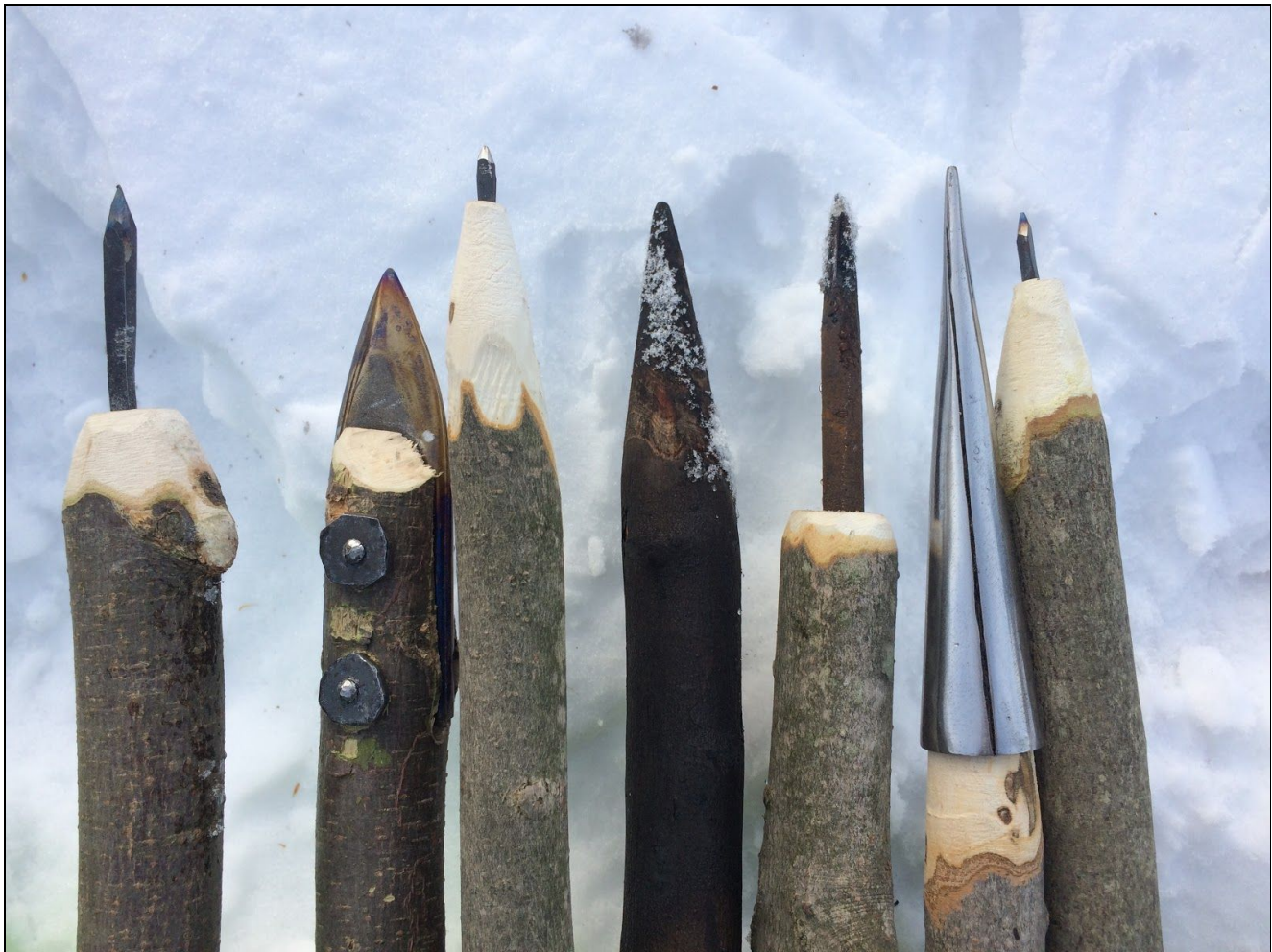
The complete set of seven pole tips. From left to right: large nail, custom mounted blade, medium nail, fire-hardened wood, hardened metal spike, spear butt cap, small nail.
