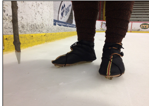
The shoes used throughout these experiments, here mounted on deer bones with leather laces.
